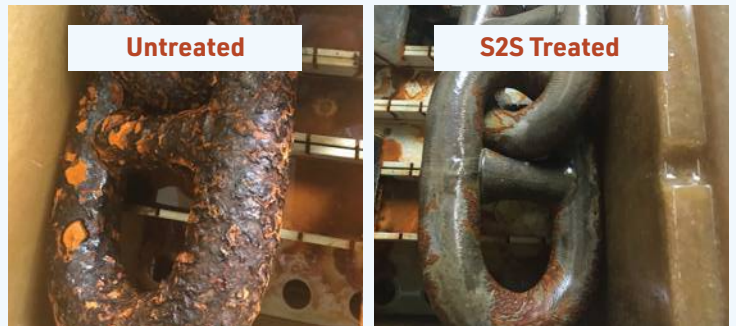
After 1000 hrs of ASTM B117 salt spray test.
