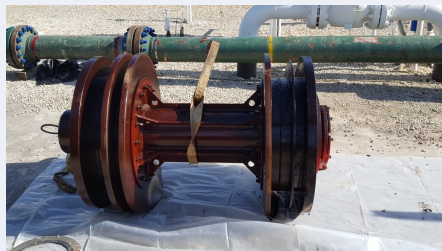
Figure 8 - Gauge pig following 2nd cleaning run (unscathed)
