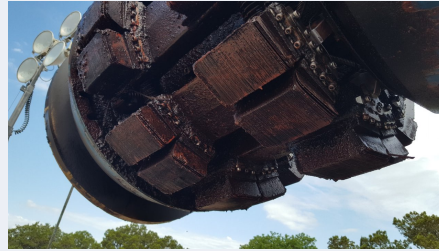
Figure 6 - Heavy Duty Cleaning Pig - T2+ Cleaning Run
