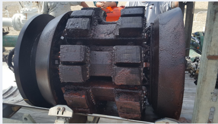
Figure 5 - Heavy Duty Cleaning Pig - T2+ Cleaning Run
