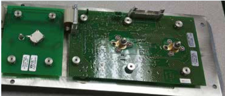
Coated with Di-Electric Spray
