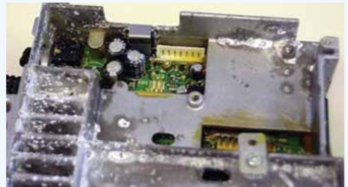
Unprotected Circuit, Heavily Corroded
