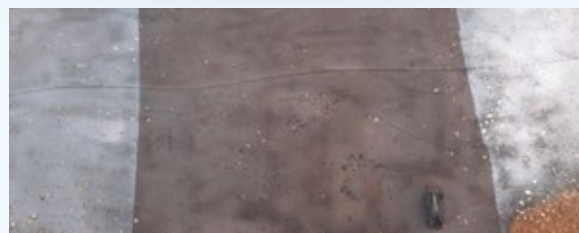
BEFORE Sandblasted white metal. Center coated in S2S
