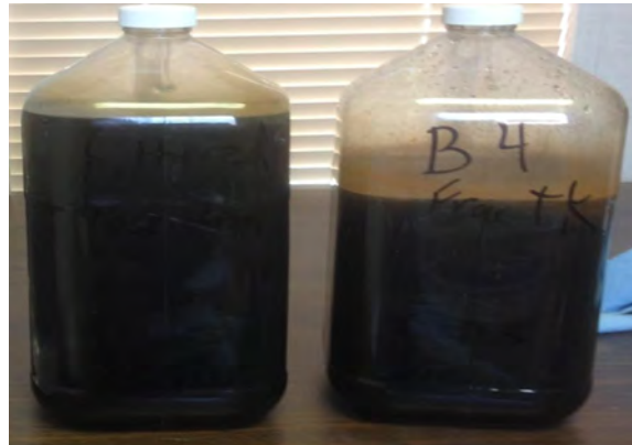
SAMPLES AFTER SRB GENERATE H 2 S
