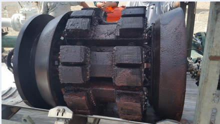
Figure 5 - Heavy Duty Cleaning Pig - T2+ Cleaning Run
