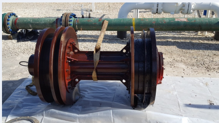
Figure 8 - Gauge pig following 2nd cleaning run (unscathed)
