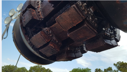
Figure 6 - Heavy Duty Cleaning Pig - T2+ Cleaning Run
