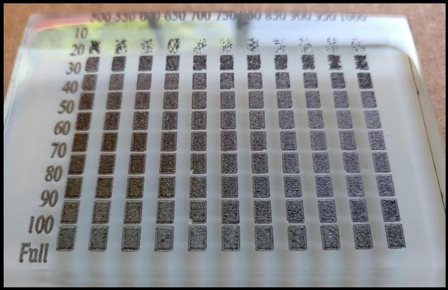
POWER on the "y" axis ↑ SPEED on the "x" axis →
