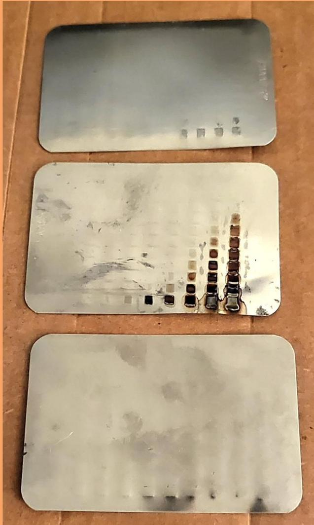
**Stainless Steel:** Lower speeds caused significant warping/damage.
