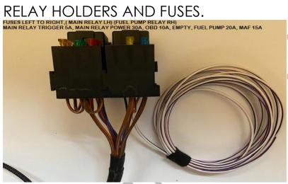
PLEASE BE AWARE FOR A RELIABLE LONG LASTING TROUBLE FREE INSTALATION IT IS PARAMOUNT THAT WIRING IS SECURLY ATTACHED TO AVOID UNDUE ABRAISION AND IS ROUTED AWAY FROM DIRECT HEAT SORCES SUCH AS TURBO CHARGERS AND EXHAUSTS.
