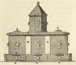
In this plate the engraver has made the floor-box to extend beyond the ends of the C. C. boxes; but, as has already been observed, and for the reason before given, it is better that the floor-box be made so that those (C. C.) boxes project a little over the ends and also over the back of the floor.
