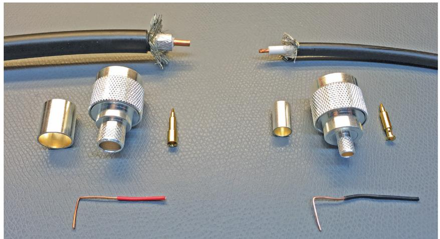
**Figure 1** — On the left, a type N crimp connector for LMR-400 coax cable and, on the right, a type N crimp connector for the thinner LMR-240 coax cable. The two L-shaped wires at the bottom are homemade stripping gauges made by inserting a piece of wire into the connector body and bending it where it stops.
