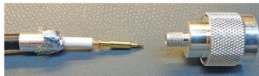
**Figure 6** — The center pin being fitted.
