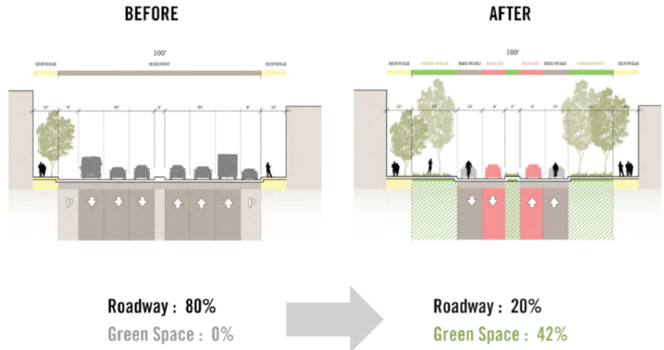
Figure 1: Diagram of 19th Avenue in San Francisco before and after AVs. Source: Gerry Tierney of Perkins and Will; presented on 5/14/2014 at SPUR San Francisco
