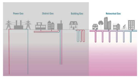
"Geothermal" is a broad term that encompasses a range of technology applications, including electricity generation (far left). The focus of this paper are the two segments on the right, shallow, low temperature geothermal. (Source: HEET)
