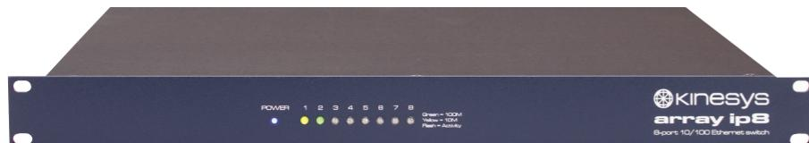
**Array IP8** is a rugged 8 port 10/100 Ethernet switch that is designed to work with Kinesys products.
