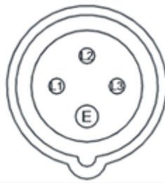
Figure 34. CEE Form IEC 60309 pinout
