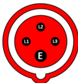
Figure 41. Red CEE form socket pinout
