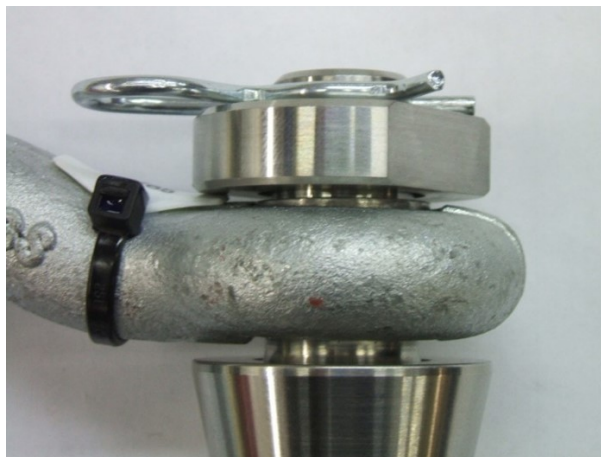
Figure 5. Nut correctly tightened
