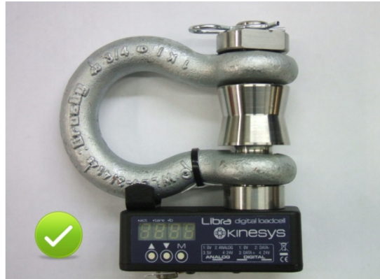
LibraCELL with Crosby shackle fitted correctly
