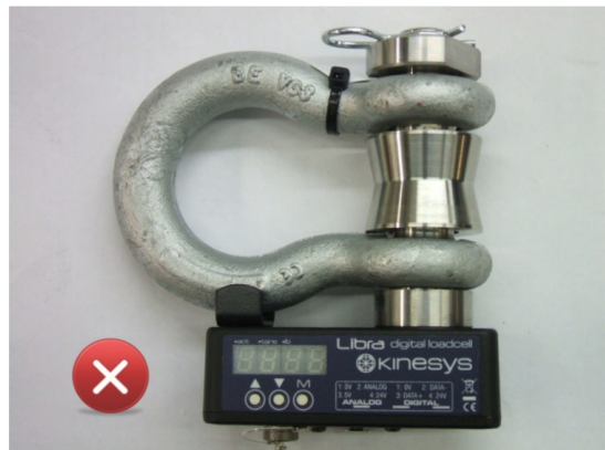
LibraCELL with Crosby shackle fitted incorrectly
