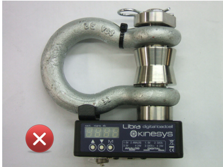
A LibraCELL with the bow fitted incorrectly.
