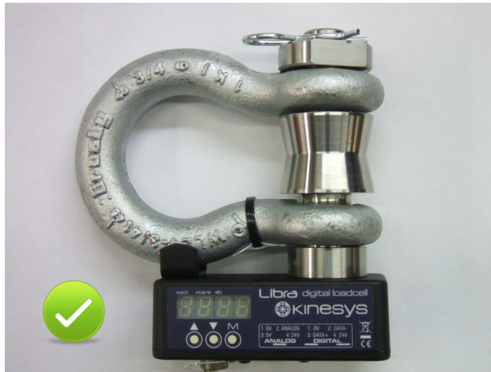
A LibraCELL with the bow fitted correctly.
