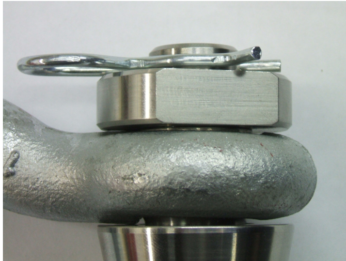
A LibraCELL with the nut correctly tightened.
