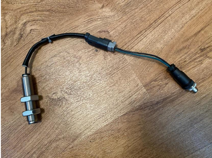
Stroke sensor and adaptor harness: NOTE: Only used on S/N 005-064
