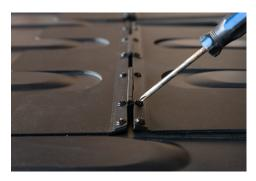
Removal: Use a #2 phillips screwdriver and firmly insert it into the screw head by tapping the top handle of the screwdriver. Then, gently unscrew without stripping the head. Additional screws are supplied if needed.
