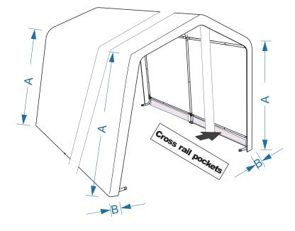
The 4 corner ropes should be in the 4 corners. When the roof tarp is in position the empty cross rail pockets should be on the side of the shelter near the ground.
