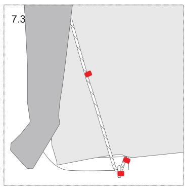
Take the cover rope under the door and hook the big loop with yellow tape to the S hook with the yellow tape on the corner upright.
