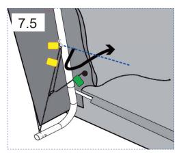
Take the black ball end of the rope, and pull the Green label up to the high smaller S hook higt . This will tighten the cover to the frame.
