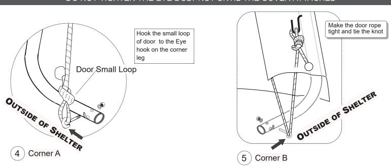
Installing the back door panel repeat process 1~5
