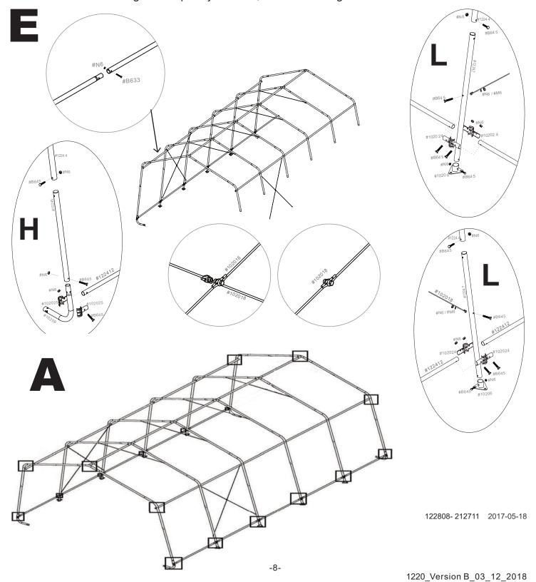
**STEP** 5: Installing the front and back door panel
