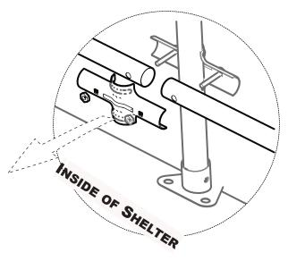
Disconnect the nuts & Rail Clamps and Bottom Rails
