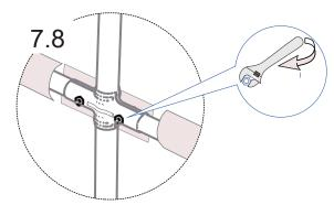
After the cover is tightened on the 4 corners with the ropes. Push and slide the bottom clamps down that are connected to the side cross rails to snug the sides of the cover to the frame. Tighten the bolts of the cross rail clamps.
