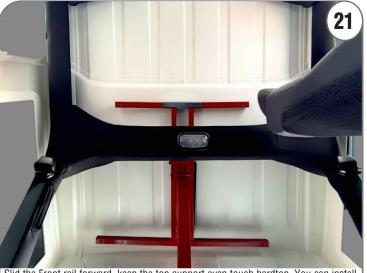
Slid the Front rail forward, keep the top support even touch hardtop. You can install provided rubber pads on top rail and high to support the hardtop even.
