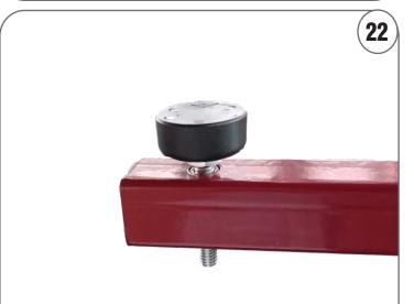
Install Rubber Pand on top rials if necessary. Be careful the don not hit the vehicle with bolts.
