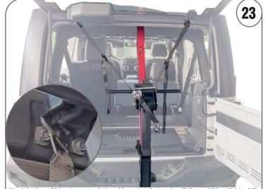
Hook both webbing to rear window hinge bracket and pull the webbing tight. Lift the Hard top off the vehicle.
