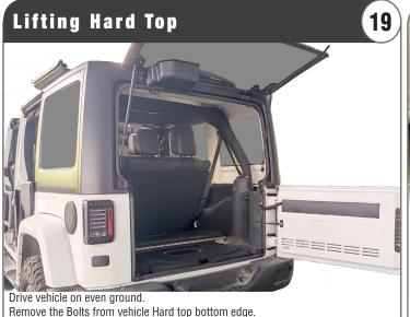
Take off the freedom Hard tops. Disconnect the wire cable, open the rear doors.
