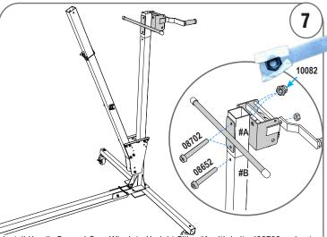
Install Handle Bar and Gear Winch to Upright Pillar #A with bolts #08702 and nuts. Install Part #A to upright pillar #B with bolts # 08652 and nuts.
