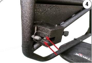
Adjust the rubber stop so the doors do not move when driving. Turn the rubber to adjust. Adjust the 2 screws if needed.
