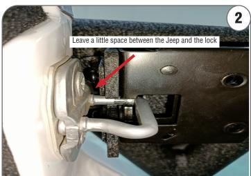
**CAUTION !** To avoid risk of injury latch mechanism must be properly adjusted before use. Inspect and adjust the door latch alignment to the door striker loop on the vehile. Check next step for adjust latch. Do not use door/latch if damaged.
