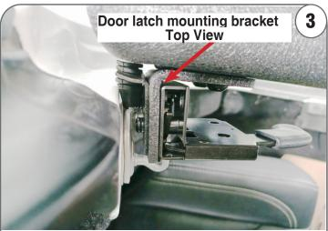
The rubber stop should not hit the jeep while adjusting.Open the latch by lift the latch handle up. Align the lock to the vehicle striker. Leave a little space between the Jeep and the lock. Make sure the lock hits the sticker in the middle. Then tighten the lock. Adjust again if needed.
