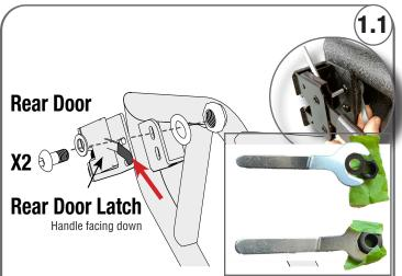
JK 2DOOR SKIP THIS STEP. Attach the rear door latch to back of the door with (2) M8x20mm bolts, (2) flat washer and (2) lock nut.DO NOT FULLY TIGHTEN hardware. Tap washer and nut on wrench to easy access back of door looking bracket.
