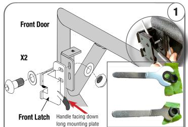
Attach the front door latch to back of the door with (2) M8x20mm bolts, (2) flat washer and (2) lock nut.DO NOT FULLY TIGHTEN hardware. Tap washer and nut on wrench to easy access back of door looking bracket.
