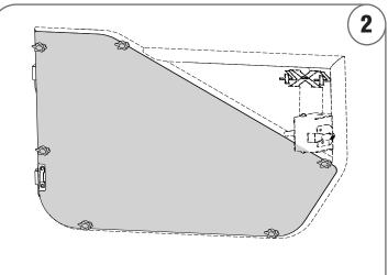
Use the thumb turn bolts to secure the panel. Store the panels so they do not rub against each other.
