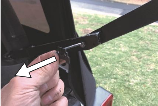
Remove the bungee and pull the pin
