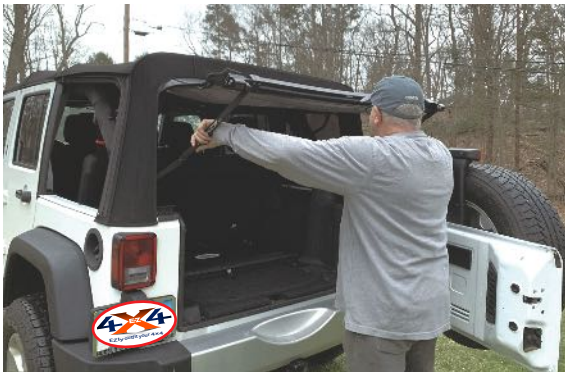
Bend the side bars up to fold the window down
