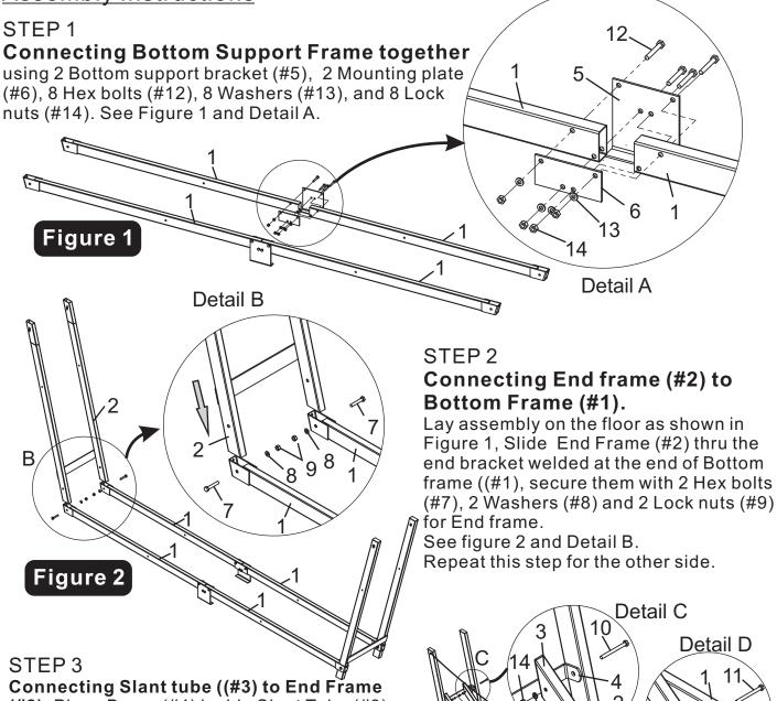
(#2). Place Brace (#4) inside Slant Tube (#3), and place Slant tube (#3) inside Brace (#4), Connect them together using 4 Hex bolts (#10), 4 washers (#13) and 4 Lock nuts (#14). See Detail C.
