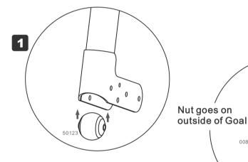
Do not over tighten the nut and bolt. It must spin inside the hole.
