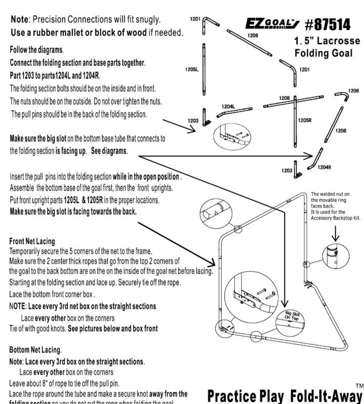
Lace the rope around the tube and make a secure knot away from the folding section so you do not cut the rope when folding the goal
