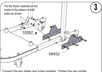
Connect the two plates and tubes together. Tighten the two middle upright tube screws. The folding outside screws should be snug not tight, so the bottom folding base swings up easily. The base should not drop down unless you pull it down.
