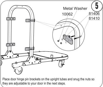
Place middle door hinge pin bracket on the upright tubes. Snug the nuts so they are adjustable to lock down your door in the next steps. The Middle bracket is a locking mechanism. This protects the doors from falling off when moving the cart.
