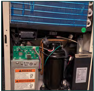
The Condensate Pump (above right) moves moisture without gravity and installs directly into the unit.
