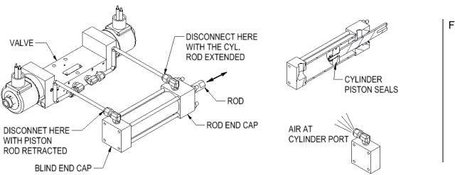
Verify if the leakage is caused by the cylinder or valve as follows: (Use extreme caution as the valve and cylinder will both be actuated during this procedure.)
