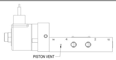
Vent leakage when the solenoid is energized can be caused by either a faulty operator piston or cap seal. Contact the factory.
