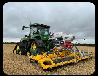
The Low Disturbance Loosener wings are hydraulically folding and can be adjusted into work and transport mode from the tractor cab. For field work, the wings unfold, interlocking into a rigid 5 or 6 metre machine and for road transport, the machine folds neatly behind the tractor and is secured with a locking bar.
