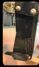
The machine is built with low disturbance legs and points which provide a full width lift with minimal surface disturbance. The front cutting disc enhances the loosening element of the leg and eliminates the surface tension thus reducing any opportunity of soil boiling in front of the leg along with easing the flow of trash through the machine.
