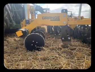
The machine wings are telescopic and have a locking position for transport. For field work the wing then slides out 0.5m to work as a 4m machine. The front cutting disc also slides inwards for transport allowing the toolbar to fit neatly behind the tractor for road use. The rear packer is hydraulically folding for transport on the 4m machine.
