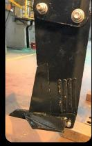
The machine is built with low disturbance legs and points which provide a full width lift with minimal surface disturbance. The front cutting disc enhances the loosening element of the leg and eliminates the surface tension, thus reducing any opportunity of soil boiling in front of the leg, along with easing the flow of trash through the machine.
