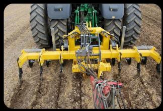
The legs are hydraulically lowered and raised without moving the main frame. This can be done on the move allowing the versatility of the loosening element of the machine in certain cultivation processes. The hydraulic front cutting discs allow complete versatility when using the machine in varying ground surface conditions especially when experiencing surface trash. This action is all achieved through one hydraulic service on the tractor.
