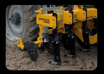
The machine wings are telescopic and have a locking position for transport. For field work the wing then slides out 0.5m to work as a 4m machine. The front cutting disc also slides in for transport allowing the toolbar to fit neatly behind the tractor for road use.
