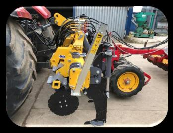
The machine is built with low disturbance legs and points which provide a full width lift with minimal surface disturbance. The front cutting disc enhances the loosening element of the leg and eliminates the surface tension thus reducing any opportunity of soil boiling in front of the leg along with easing the flow of trash through the machine.
