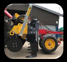
The machine has a depth of 912mm from couple point to the rear link arms on the toolbar, keeping overall length down for manoeuvrability.
