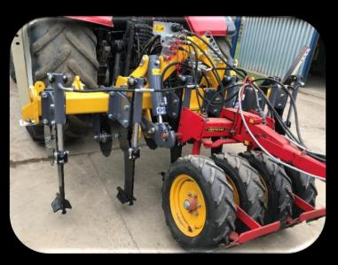
The close coupled toolbar is lowered in and out of work simply using the three point linkage on the rear of your tractor, using position control you can then set your required working depth of the low disturbance leg. The rear link arms operate via hydraulic operation so that the implement behind can maintain the same working depth even when the toolbar is lifted out of work.
