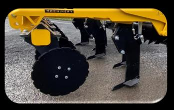
The machine is built with low disturbance legs and points which provide a full width lift with minimal surface disturbance. The front cutting disc enhances the loosening element of the leg and eliminates the surface tension thus reducing any opportunity of soil boiling in front of the leg along with easing the flow of trash through the machine.
