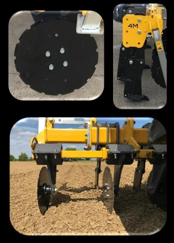
The machine is fitted with Grange low disturbance legs and points which provide a full width lift with minimal surface disturbance. The front cutting disc enhances the loosening element of the leg and eliminates the surface tension thus reducing any opportunity of soil boiling in front of the leg along with easing the flow of trash through the machine.
