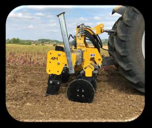
The machine has a depth of 912mm from tractor couple point to the rear link arms on the toolbar, keeping overall length down for manoeuvrability.
