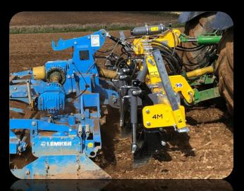
The Close Coupled Toolbar is lowered in and out of work simply using the three point linkage on the rear of the tractor, using position control you then set the required working depth of the low disturbance leg. The rear link arms operate via hydraulic operation allowing the trailed/mounted implement to maintain the same working depth even when the toolbar is lifted out of work.
