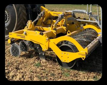
The 6 Metre Low Disturbance Loosener wings are hydraulic folding and can be adjusted into work and transport mode from the tractor cab. For field work, the wings unfold, interlocking into a rigid 6 metre machine and for road transport, the machine folds neatly behind the tractor and is secured with a locking bar.
