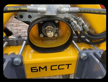
The Close Coupled Toolbar is lowered in and out of work simply using the three point linkage on the rear of the tractor, using position control you then set the required working depth of the low disturbance leg. The rear link arms operate via hydraulic operation allowing the trailed/mounted implement to maintain the same working depth even when the toolbar is lifted out of work.
