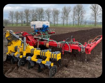
The machine is fitted with Grange low disturbance legs and points which provide a full width lift with minimal surface disturbance. The front cutting disc enhances the loosening element of the leg and eliminates the surface tension thus reducing any opportunity of soil boiling in front of the leg along with easing the flow of trash through the machine.
