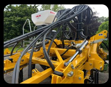
A unique feature of the design is the use of contouring wings which have a pivot pitch of up to 5deg side to side integrated into the carrying frame above each wing to allow for undulations and varying terrain, maintaining seed depth from front to back and across the full width of the drill.
