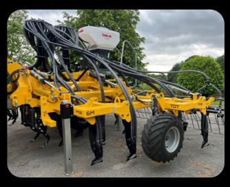
The frame is supplied with a CAT3 and 4 linkage headstock and uses 20mm Grange tines over four rows on the toolbar frame at a tine spacing of 250mm centres featuring a resting area in the centre section for optimum trash flow management
