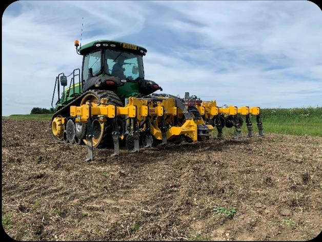
The machine wings are hydraulic and can be folded into work and transport position from the tractor cab. For field work the wings fold downwards interlocking into the main frame to work as a 6m machine. The front cutting disc fold for transport allowing the toolbar to fit neatly behind the tractor for road use.
