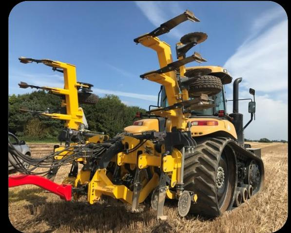
The '**Tight – Turn**' system on the 6m toolbar ensures that the wings fold upward to 90 degrees automatically when the legs are hydraulically lifted out of work. This movement creates space for the operator to turn close to the trailing implement allowing for a 'Tight Turn' to be achieved on headlands.
