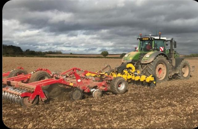
The legs and cutting discs are hydraulically lowered and raised without moving the main frame. This can be done on the move allowing the versatility of the loosening element of the machine in certain cultivation processes. Both legs and discs work using one hydraulic service. This system allows the discs to cut deeper in ratio to the legs working deeper.
