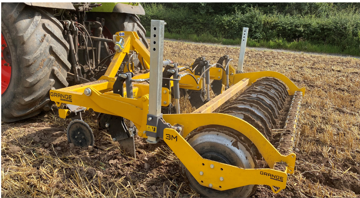
FIG 7.0 GRANGE 3M GLL IN THE WORKING POSITION
