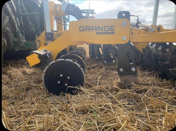
The machine wings are telescopic and have a locking position for transport. For field work the wing then slides out 0.5m to work as a 4m machine. The front cutting disc also slides inwards allowing the toolbar to fit neatly behind the tractor for transport. The rear packer is hydraulically folding for transporting the 4m machine.
