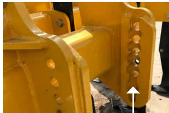
FIG 10.0 LINK ARM HITCH REMOVED FROM REAR OF GRANGE 4M LDT
