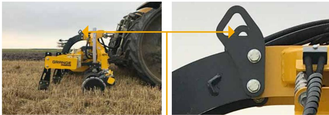
FIG 1.0: LIFTING AND SLINGING POINTS
