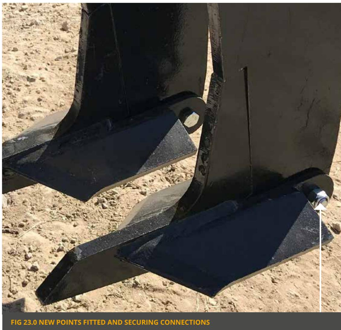
FIG 23.0 NEW POINTS FITTED AND SECURING CONNECTIONS
