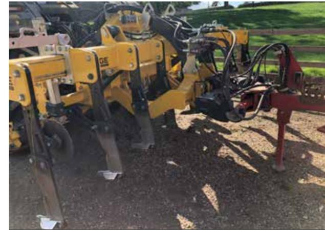
FIG 6.0 4M LDT IN COUPLING POSITION WITH 2ND STAGE CULTIVATION EQUIPMENT
