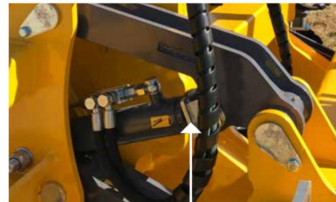
FIG 19.0 LOCATION FOR LIFT AND LOWER DISC RAM DEPTH SPACERS
