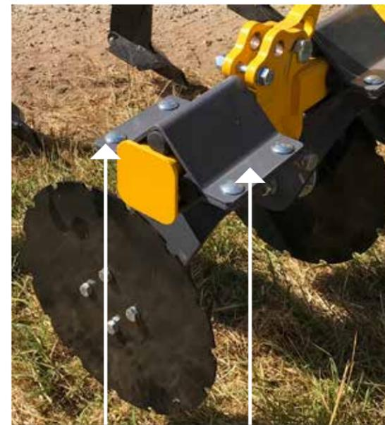
FIG 11.0 LIFTING POINTS FOR MANUAL ADJUSTING DISC WING SECTION.
