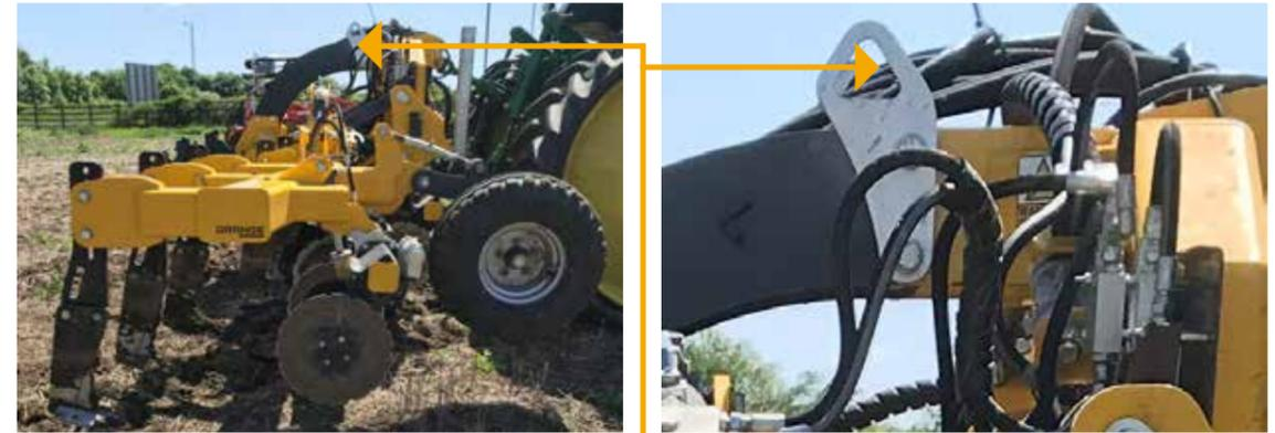
FIG 1.0: LIFTING AND SLINGING POINTS
