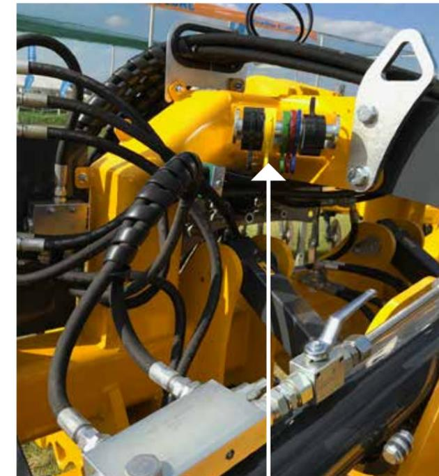
FIG 3.0 LIFT AND LOWER RAMS - DEPTH CONTROL
