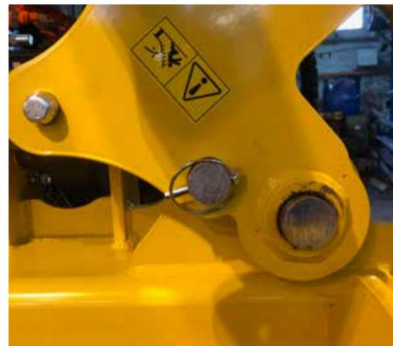
FIG 18.0 TIGHT TURN PIN SECURING THE WING IN POSITION WITH LYNCH PIN. VIEW FROM REAR OF GRANGE 6M LDT
