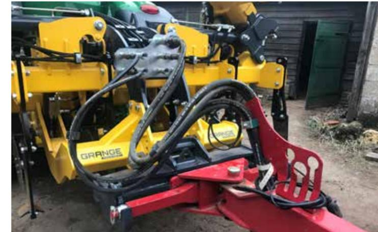
FIG 6.0 6M LDT IN COUPLING POSITION WITH 2ND STAGE CULTIVATION EQUIPMENT
