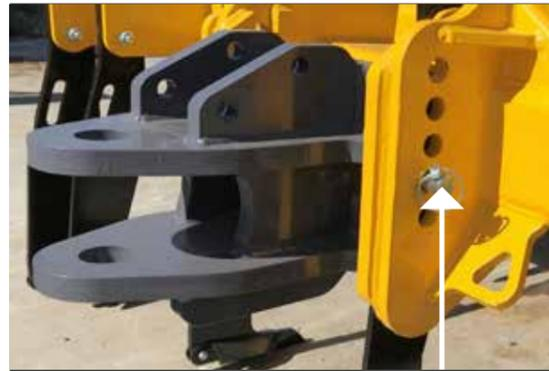
FIG 8.0 LYNCH PIN FOR SECURING ATTACHMENT PIN
