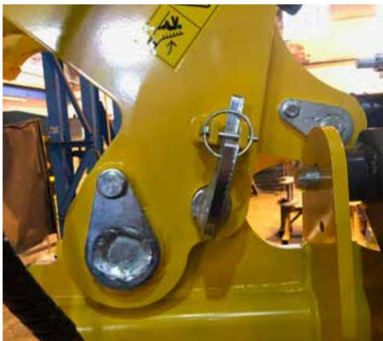
FIG 17.0 TIGHT TURN PIN SECURING THE WING IN POSITION WITH LYNCH PIN- FRONT VIEW FROM TRACTOR LINKAGE
