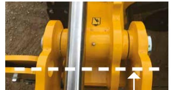
FIG 12.0 TIGHT TURN PIN REMOVED FROM WING
