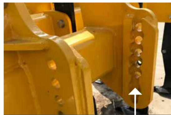
FIG 10.0 LINK ARM HITCH REMOVED FROM REAR OF GRANGE 6M LDT
