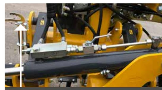
FIG 13.0 TIGHT TURN PIN STOWED ON FRAME
