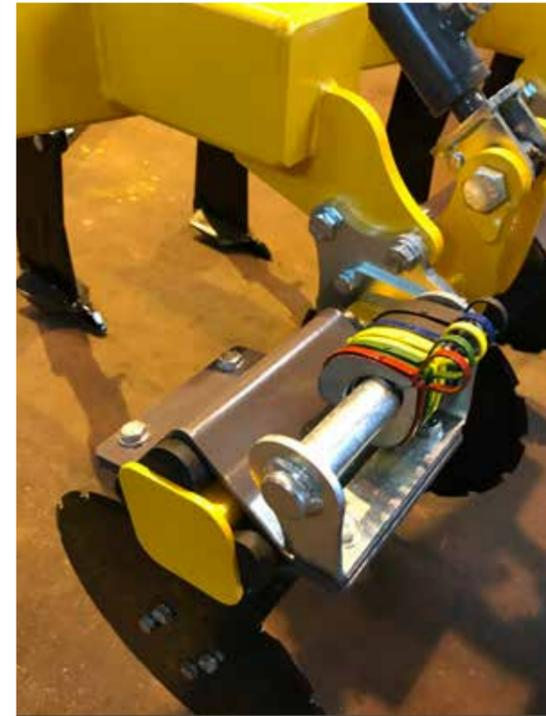
FIG 19.0 DEPTH SPACERS FOR DISC RAM IN STORAGE POSITION.
