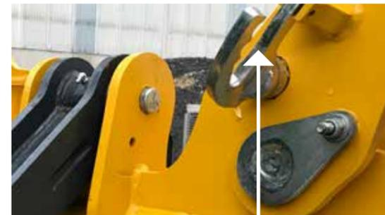
FIG 11.0 REMOVE TIGHT TURN PIN FROM WING
