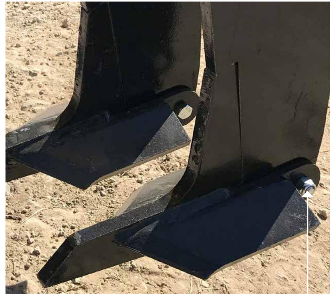
FIG 17.0 NEW POINTS FITTED AND SECURING CONNECTIONS
