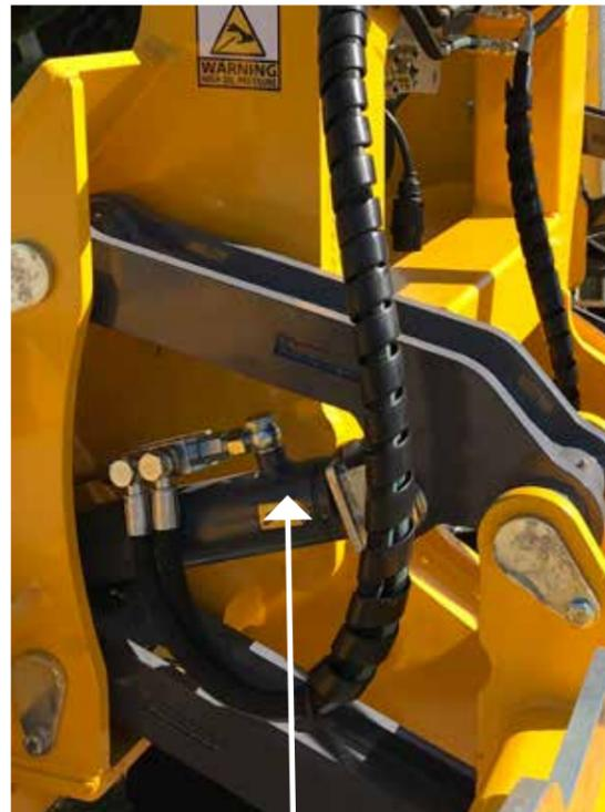
FIG 13.0 LOCATION OF DEPTH SPACERS ON MAIN BEAM RAM
