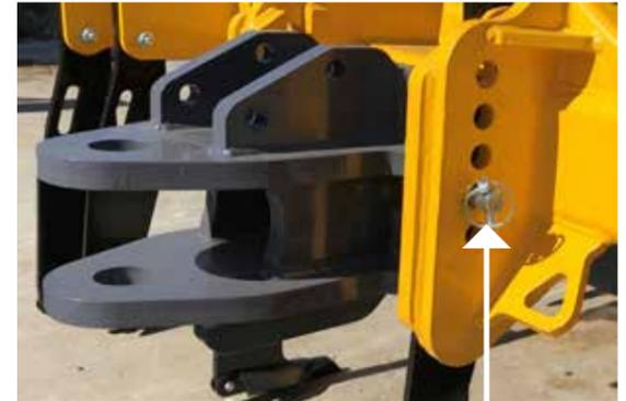
**FIG 8.0 LYNCH PIN FOR SECURING ATTACHMENT PIN**
