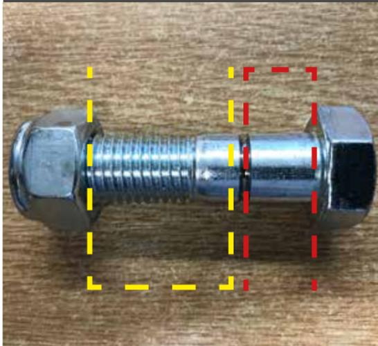
FIG 15.0 SHEAR BOLT WITH SHEAR PLANE
