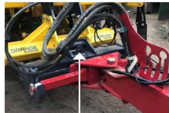
**FIG 9.0 SECURING POINT FOR LINK ARM HITCH REMOVAL**
