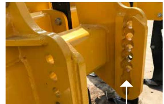
**FIG 10.0 LINK ARM HITCH REMOVED FROM REAR OF GRANGE 3M LDT**
