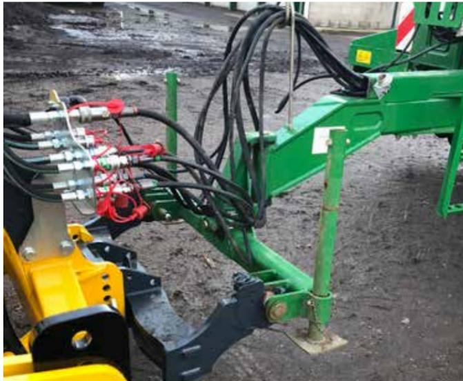
**FIG 6.0 3M LDT IN COUPLING POSITION WITH 2ND STAGE CULTIVATION EQUIPMENT IN WORKING MODE**
