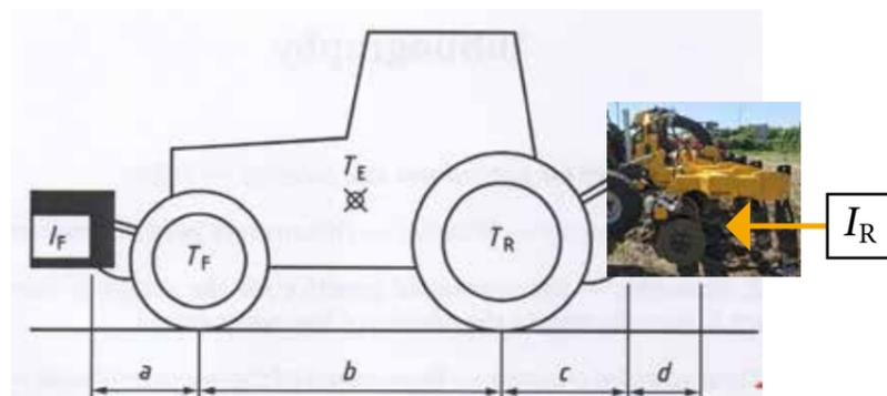
$$I_{F, \min} = \frac{(I_R \times (c+d)) - (T_F \times b) + (0,2 \times T_E \times b)}{a+b}$$
