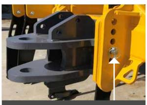
FIG 8.0 LYNCH PIN FOR SECURING ATTACHMENT PIN
