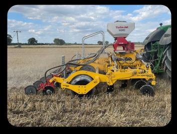
The 4 Metre Low Disturbance Loosener wings are hydraulic folding and can be adjusted into work and transport mode from the tractor cab. For field work, the wings unfold, interlocking into a rigid 4 metre machine and for road transport, the machine folds neatly behind the tractor and is secured with a locking bar.
