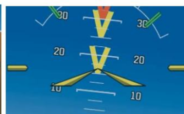
ESP Roll Engagement Indication (ESP Enabled but NOT Engaged)
