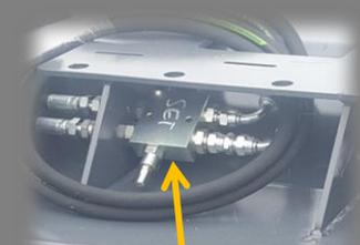
Plumbed / remote hydraulic located relief valve
